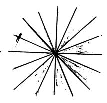
All lines should come together this way and you have the center marked for you. Using a four jaw chuck on your lathe, turn the end round at the tail stock. Now take the part and turn it around and mount in a three jaw chuck. Finish turning so that you end up with a straight cylinder.
