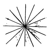
All lines should come together this way and you have the center marked for you. Using a four jaw chuck on your lathe, turn the end round at the tail stock. Now take the part and turn it around and mount in a three jaw chuck. Finish turning so that you end up with a straight cylinder.
