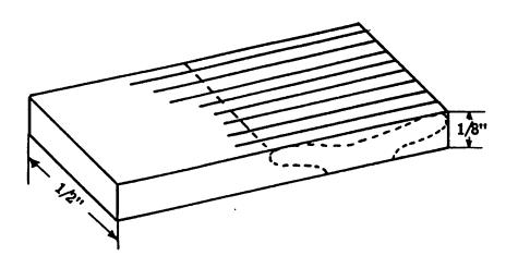
By holding the base of the blank in a pair of squarenose pliers, the horns may be rounded with a needle file and desired shape smoothed with fine sandpaper.
