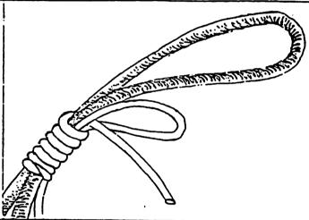
Step 4. Place the working end through the loop formed in step 2.
