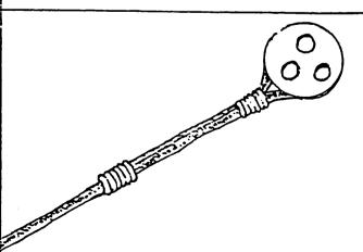
Step 6. Slide the sieze to where it is needed, insert Deedeye and pull the excess line through the sieze. until the Deadeye is captured. Cut excess line.
