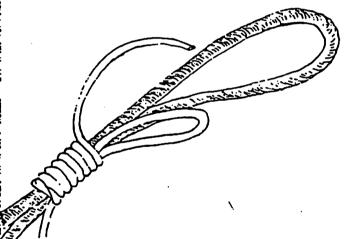
Step 3. With the working end, begin wrapping. Keep the coils close together. Keep count of the number of turns so later siezes are the same size.
