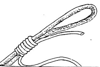
Step 5. Pull the spool end, pulling the working end under the coils. Pull both ends against one another to make the sieze tight.
