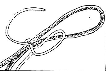
Step 2. Make a loop with the spool end laying the loop intersection on the intersection of the overhand knot.
