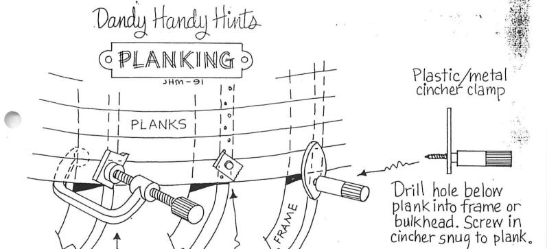
There are many styles & sizes of "C" clamps. Use a small scrap of soft wood to prevent clamp from denting plank.
