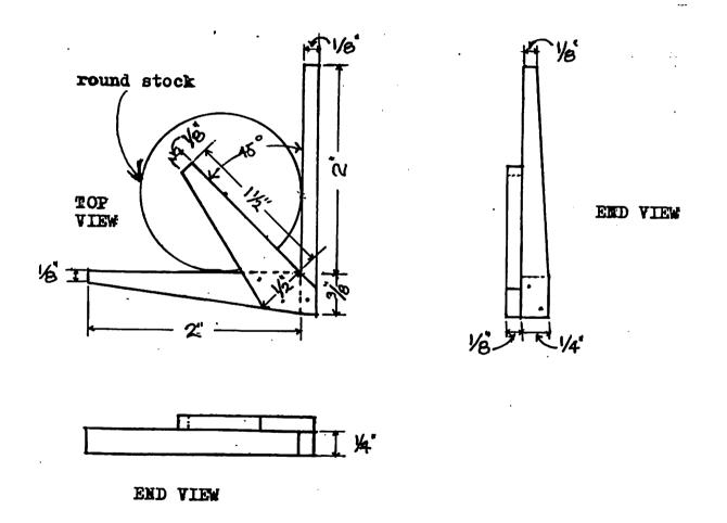
The material used should be hardwood such as birch or maple. After gluing together I used 1/4" brads to make secure. Be sure that the L piece is absolutly square, and the diagonal piece is exactly at 45 deg..
