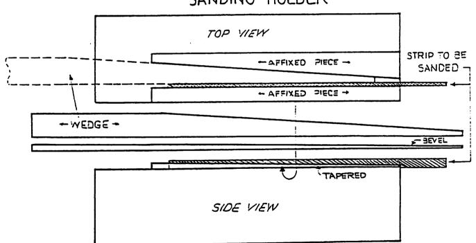
For holding those small parts for sanding-such as hull planks that you want to taper to the stern or stem posts.
