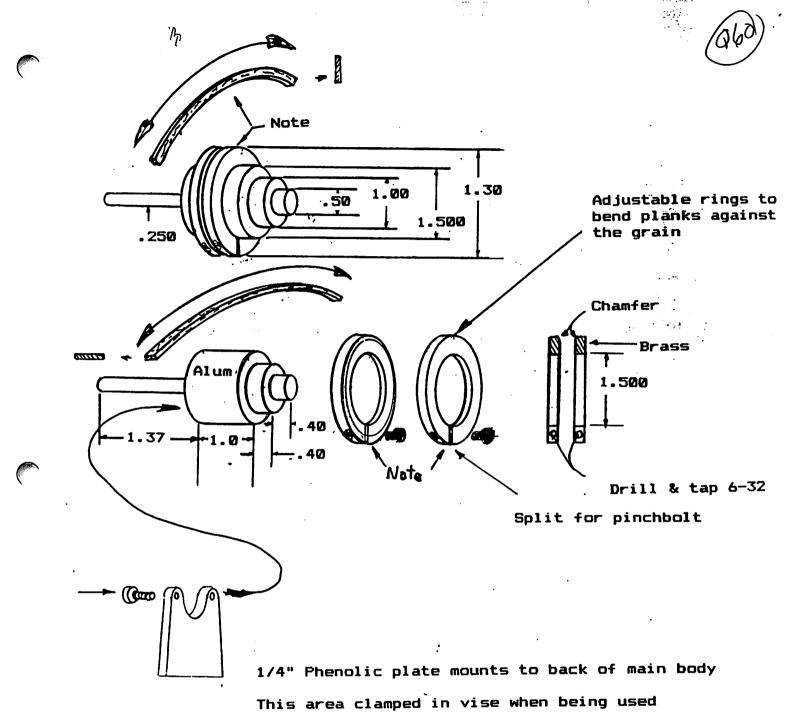
Plank bending device for bending planks either with the grain or against the grain.
