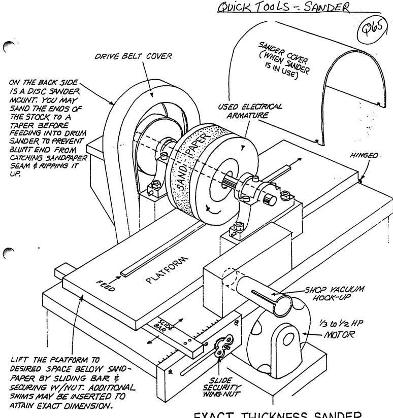
EXACT THICKNESS SANDER Excellent for precise hull/deck planking plus other uses.
